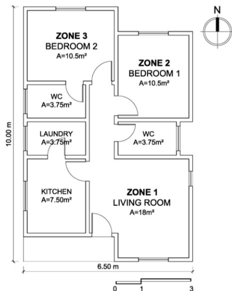
Figure 3 – Floor plan of the baseline model.
