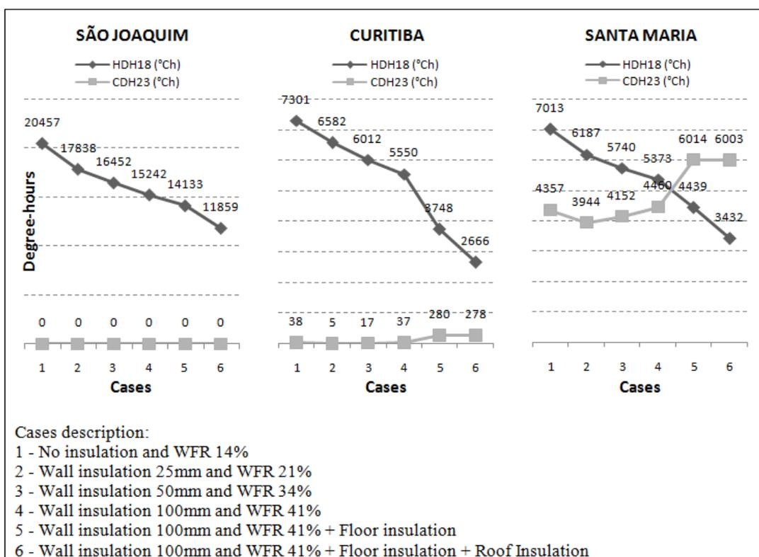
Figure 2 – Modeling optimization results from the third step of sensitivity analysis.
